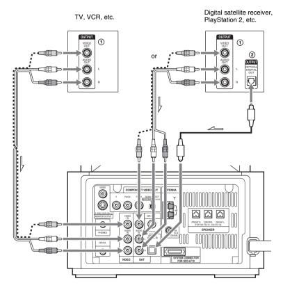
Connect the AUDIO OUT (L/R) jacks (①) to the VIDEO or SAT AUDIO IN (L/R) jacks of this subwoofer with audio cords (not supplied). If your TV does not have the AUDIO OUT (L/R) jacks, you cannot output the TV sound from the speakers of this subwoofer. If your TV has an OPTICAL DIGITAL OUT jack (②), connect to the SAT OPTICAL DIGITAL IN jack of this subwoofer using an optical digital cord (not supplied).
